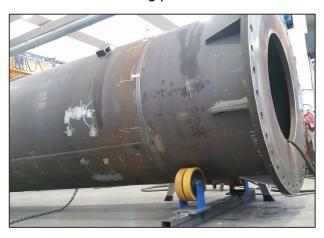
This solution allows to realize structures that are shaped by following the trend of the moments and forces (dynamic loads applied); also allow the use of *greater thickness where it is needed and smaller thicknesses where the material is less stressed*, moreover this type of construction, plans to enter the <u>internal baffles</u> to increase the rigidity of the structure in particular in the way the points of application of the load.
