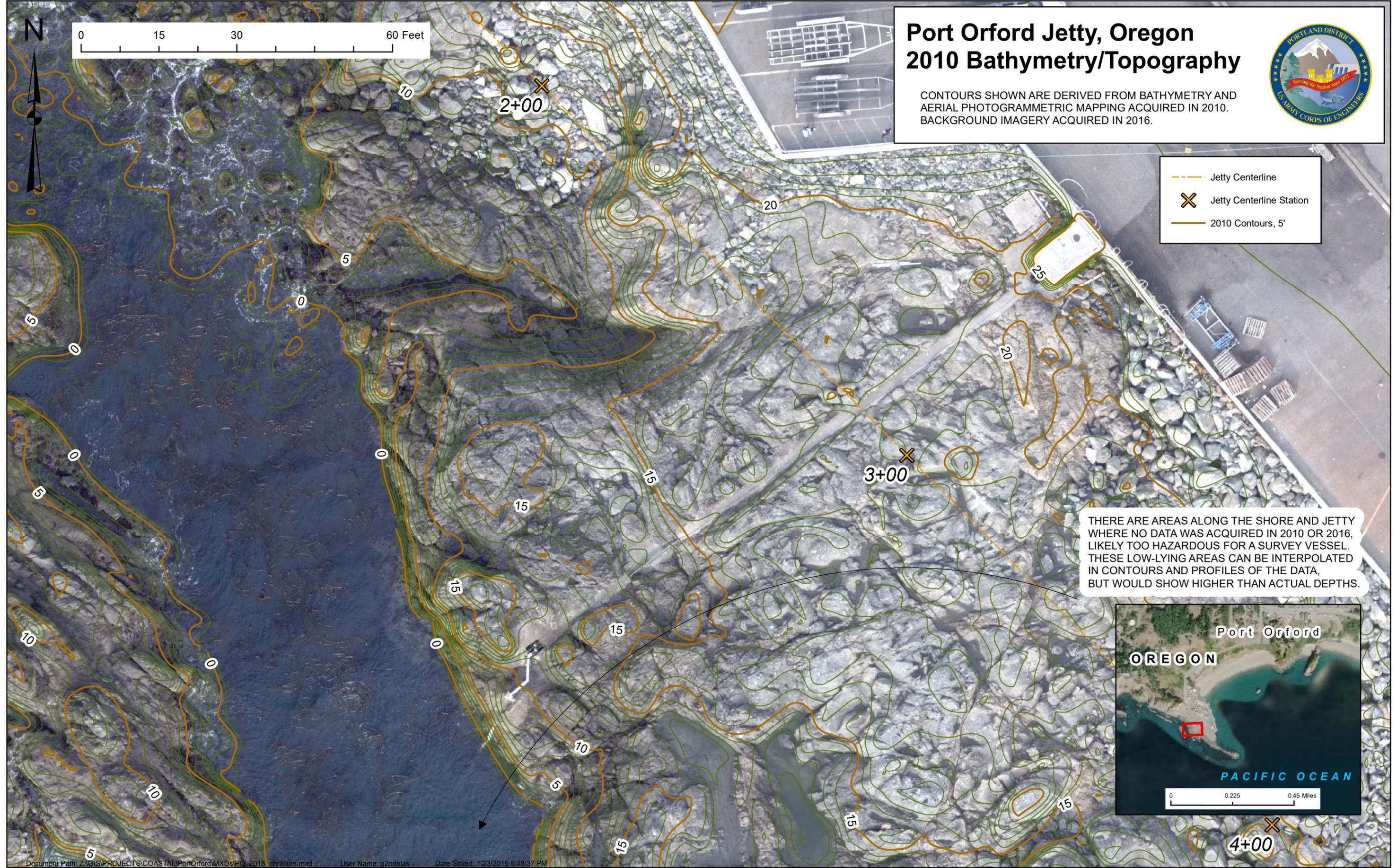
THERE ARE AREAS ALONG THE SHORE AND JETTY WHERE NO DATA WAS ACQUIRED IN 2010 OR 2016, LIKELY TOO HAZARDOUS FOR A SURVEY VESSEL. THESE LOW-LYING AREAS CAN BE INTERPOLATED IN CONTOURS AND PROFILES OF THE DATA, BUT WOULD SHOW HIGHER THAN ACTUAL DEPTHS.
